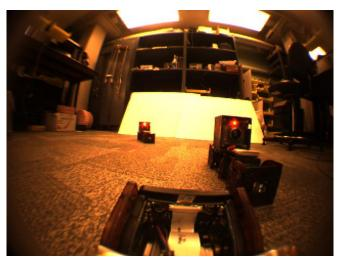
Fig 4: A view of the two other legs from the torso camera module. The wide angle fish-eye lens covers almost 240 degree.
