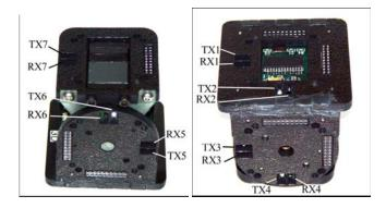
Fig. 2: Two IR transmitter and receiver pairs are on each side of a CKbot module except the bottom port which has one pair.
