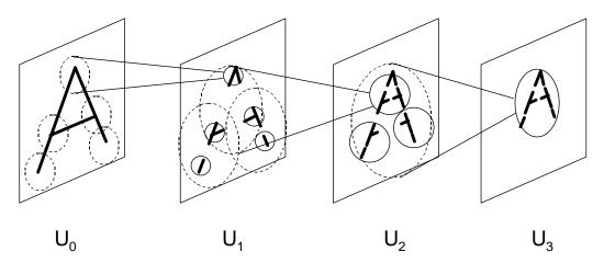
Figure 2.5 Neocognitron model of pattern recognition (adapted from Fukushima [8] and slightly modified).
