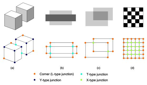
Figure 2.1 Schematic explaining how different types of junctions are generated in different configurations of objects. For each image, junctions are superimposed on an edge-extracted image shown below the corresponding original image. (a) Three-dimensional view of two cubes. The front one occludes the rear one. (b) Two sheets in which an opaque one is placed on top of the other. (c) Two sheets in which a transparent one is placed on top of the other. (d) Checkerboard pattern.
