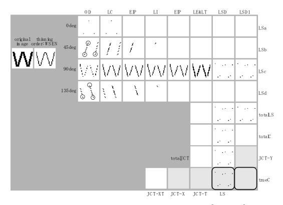
Figure 2.29 Simulation result for letter "W". The line segments in  $45^{\circ}$  and  $135^{\circ}$  orientations constituting the three corners (shown in the circle) are removed by the EIP operation since the line length is two. This result in the failure of corner detection; linestops are detected instead (shown in the rectangle of a thick boundary).
