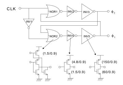
Figure 5.12 Schematic of the two-phase clock generator.
