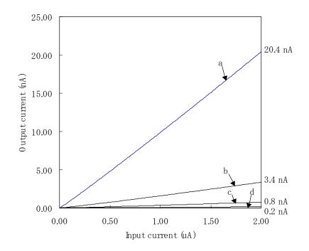
Figure 3.8 Relationship between the input current and the output current for different switch settings for the circuit shown in Figure 3.7. The value shown at the right end of the line indicates an output current for the input current of 2  $\mu$ A.
