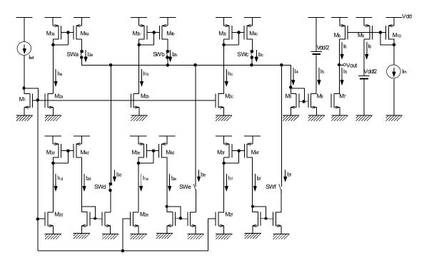
Figure 4.8 Current thresholding circuit as an example to demonstrate the design procedure. The thresholding scheme is slightly different from the one shown in Figure 3.9.
