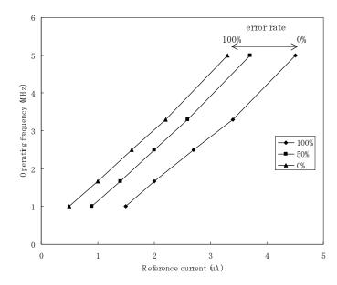
Figure 5.25 Variation of the operating frequency for different error rates. The experiment was conducted for the maximum delay of 35.4 nsec.
