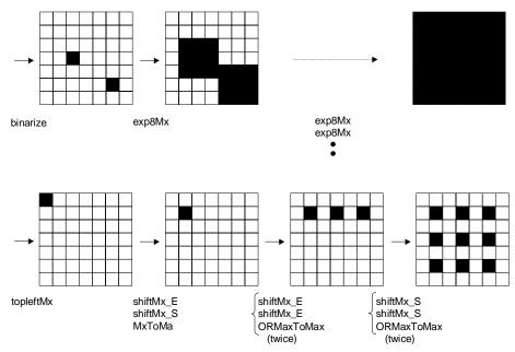
Figure 5.21 Method of generating a grid pattern. It is explained for a small matrix of  $7 \times 7$  instead of  $16 \times 16$  for simplicity. The operation necessary for image transformation is shown below the arrow.
