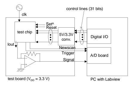
Figure 5.18 Schematic of the connection between the test board which contains the test chip and the PC equipped with a digital I/O board and an A/D converter.
