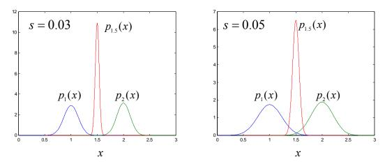
Figure 4.9 Probability distributin function of the output current and the threshold current for different relative current variations (left: s=0.03; right: s=0.05). Note that the x-axis is scaled to  $I_{ref}$ .  $p_1(x)$  and  $p_2(x)$  represents the output current distribution for the current whose mean is  $I_{ref}$  and  $2I_{ref}$ , respectively.  $P_{1.5}(x)$  represents the distribution of the threshold current whose mean value is  $1.5I_{ref}$ .
