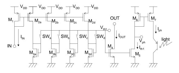
Figure 3.7 Schematic of image digitization circuit with an adjustable threshold current. The transistor sizes (*W/L*) are as follows:  $M_1$ ,  $M_{2a}$ ,  $M_{2b}$ ,  $M_{2c}$ ,  $M_{2d}$ ,  $M_6$ ,  $M_7$ : 1.5/2.7;  $M_{3a}$ : 9/0.9;  $M_{3b}$ : 30/0.9;  $M_{3c}$ : 90/0.9;  $M_{3d}$ : 300/0.9;  $M_4$ ,  $M_5$ : 1.5/4.2.
