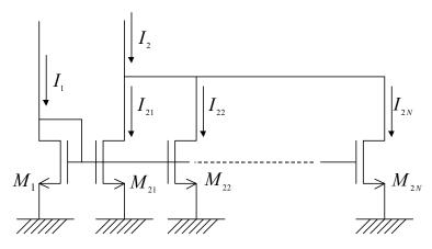
Figure 4.6 Generalized current summation circuit. Note that correlation exists between  $I_{21}$ ,  $I_{22}$ , ...,  $I_{2N}$ .
