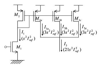
Figure 4.5 The other type of current summation circuit. Note that correlation exists between three current outputs  $I_{3a}$ ,  $I_{3b}$ , and  $I_{3c}$ .
