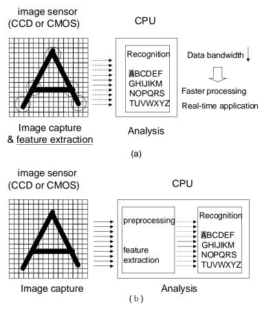
Figure 1.2 Two types of pattern recognition systems. (a) Newly proposed pattern recognition system using the feature detection sensor as a front-end. (b) Conventional pattern recognition system. Note that the feature extraction carried out in a CPU in (b) is incorporated inside the sensor in (a).
