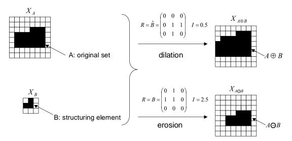
Figure 2.12 Example of dilation and erosion. The original set *A* is processed with the structuring element *B* to produce the dilated and eroded set. The origin of the structuring element is defined at the center of the  $3 \times 3$  region. The combination of the template and the threshold to carry out these two operations are also listed in the figure.
