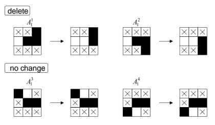
Figure 2.15 Algorithm for thinning. A pixel is deleted if its  $3 \times 3$  neighbors match either  $A_1^1$  or  $A_1^2$  and match neither  $A_1^3$  nor  $A_1^4$ .
