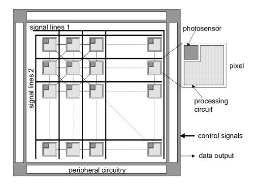
Figure 3.1 General architecture of vision sensors. A rectangular array of pixels, each of which consists of the photosensor and the processing circuit, and the peripheral circuit constitute the vision sensor. The sensor receives a set of control signal and produces an output.
