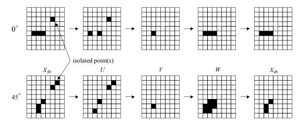
Figure 2.21 Procedure of *elimination of isolated points* operation in  $0^{\circ}$  orientation (top) and in  $45^{\circ}$  orientation (bottom).
