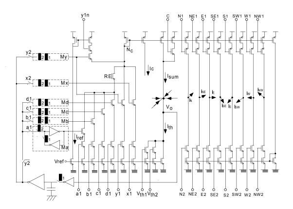
Figure 3.9 Schematic of the processing circuit.
