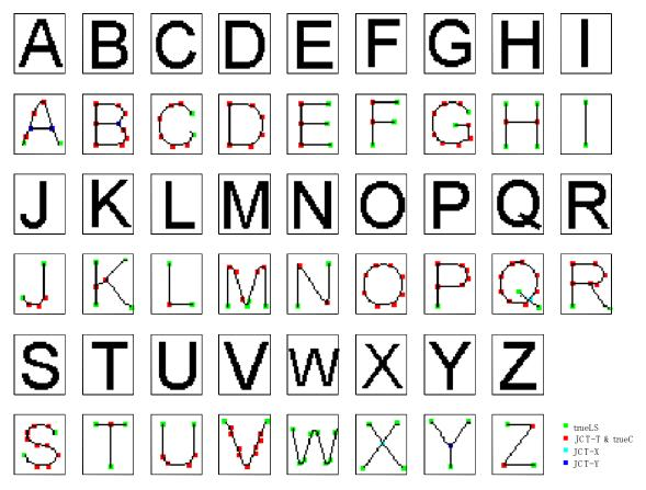
Figure 2.27 Features detected by the proposed algorithm for alphabetical characters. The center of a closed rectangle indicates the position of a feature. The shade of the rectangle represents the type of the feature.
