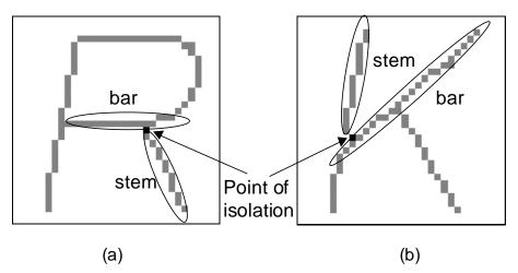
Figure 2.31 Pixel point where the stem is separated from the bar of the T-type junction for two letters "R" and "K". It is superimposed on the original letter displayed with half-tone color. (a) The local orientation of this point is computed as  $90^{\circ}$ . (b) No orientation is assigned to this point.
