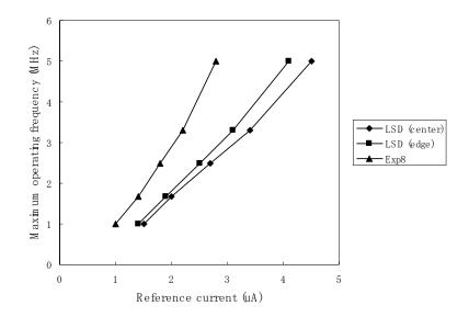
Figure 5.26 Maximum operating frequency for three types of operations. The experiment was conducted for the maximum delay of 35.4 nsec. The error for the Exp8 operation is defined as the generation of a pixel of value 1 by the application of this operation for an entire array of pixels of value 0.
