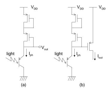
Figure 3.4 Logarithmic compression circuit. (a) Mahowald and Mead's logarithmic compression circuit [9]. (b) Etienne's compression circuit with an additive transistor to produce an amplified current output [7].
