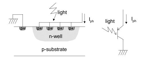
Figure 3.3 Structure of the phototransistor. The phototransistor is formed vertically by defining p+ emitter region in the n-well. The n-well serves as the base while the p-substrate works as the collector. The emitter region is defined in a stripe manner for allowing the light to easily reach the base region.
