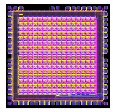
Figure 5.17 Layout of the entire chip.
