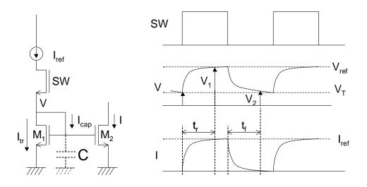
Figure 4.11 Schematic to explain the charging and discharging of the capacitance associated with the gate. The rise time  $t_r$  is defined as the time for the current to reach 95% of  $I_{ref}$  while the fall time  $t_f$  is defined as the time for the current to reach 5% of  $I_{ref}$ .
