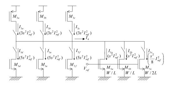
Figure 4.14 Extracted schematic from Figure 3.9 focusing on the current thresholding node. Expression in a parenthesis represents the variance of the current shown above the parenthesis.
