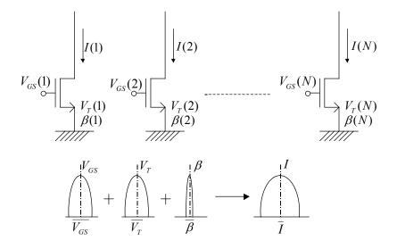
Figure 4.2 Variation of the output currents from a set of transistors with different gate voltages and process parameters. Note that Figure 4.1 is a special case where the gate voltage is common for all transistors.
