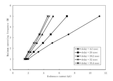
Figure 5.24 Maximum operating frequency as a function of the reference current for different settings of internal delay between  $\phi_2$  and  $\phi_{2d}$ . The experiments were carried out to find the minimum required current for certain frequencies. The maximum frequency was 5 MHz due to device limitation.
