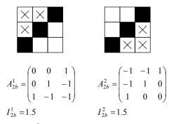
Figure 2.18 Patterns categorized as  $45^{\circ}$  with its corresponding template and threshold.
