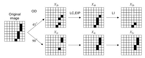
Figure 2.22 Procedure of line inhibition operation.
