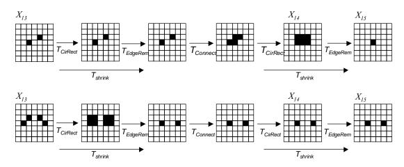
Figure 2.26 Merging of linestops which originally belong to different orientation planes.
