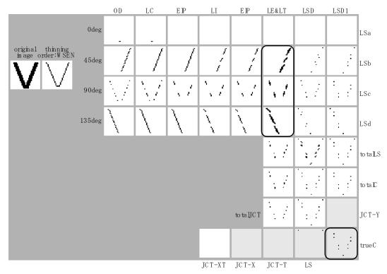
Figure 2.28 Simulation result for letter "V". Each of the two diagonal line segments is represented as an alternating sequence of  $45^{\circ}$  and  $90^{\circ}$  line segments, resulting in unexpected corners (shown in the rectangle of a thick boundary).
