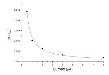
Figure 5.22 Relative variation of the current as a function of the reference current.
