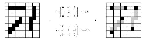
Figure 2.10 Linestop detection based on template matching. The combination of the template and the threshold shown above the arrow is equivalent to the combination of the template and the threshold shown below the arrow.
