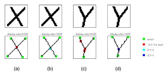
Figure 2.33 Effect of thinning order on the feature detection. Thinning was performed in the order of west, south, east, and north for (a) and (c), while it was performed in the order of south, east, north, and west for (b) and (d).
