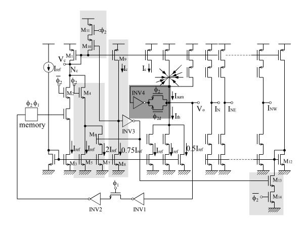
Figure 5.7 Pixel circuit incorporating the second mechanism for high speed operation. The dark shaded block is implemented to keep the voltage of the thresholding node constant before starting the current mode processing.
