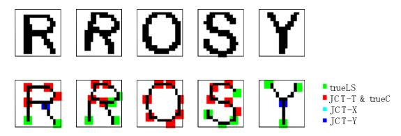
Figure 5.27 Sensor responses to various letter images. For an input image shown on the top row, a set of features is obtained as shown in the bottom row. These features are superimposed on the thinned image. The center of a closed rectangle indicates the position of the detected feature.
