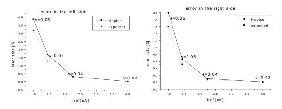
Figure 4.15 Expected and simulated error rate as a function of the reference current. The dashed line represents the expected error rate, while the solid line represents the Monte-Carlo simulation result using Hspice circuit simulator.
