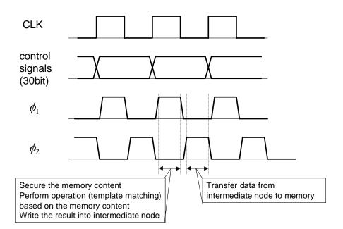
Figure 3.10 Timing diagram for chip operation. The function associated with each phase is described in the box. The control signals consists of those shown in Figure 3.9 (a1, b1, ..., NW1, NW2). The two-phase clock ( $\phi_1$  and  $\phi_2$ ) are generated from CLK.
