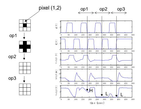
Figure 5.6 Simulation results at the clock frequency of 10 MHz using the modified circuit incorporating the high speed charging/discharging mechanism. An error was observed for op1 operation at the pixel (1,2). The voltages and the current on the right-hand waveforms represent those at the pixel (1,2).
