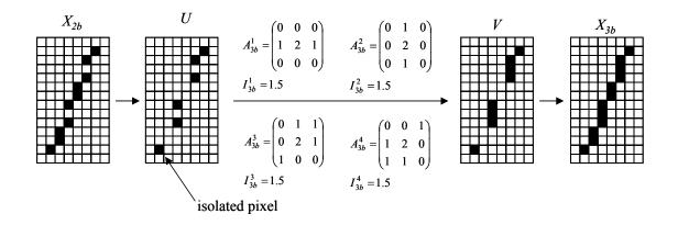
Figure 2.20 Procedure of *line completion* operation in  $45^{\circ}$  orientation. Four templates used to obtain image *V* from *U* are shown above and below the arrow.
