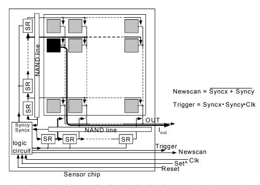
Figure 5.14 Schematic of the scanning circuit. The pixel is connected to the output through two switches: the black pixel is connected to the output through a thick line above. The switches are controlled by the output of the shift register, which transfers logic Low. Scanning is carried out in an autonomous way by automatically generating logic Low when the outputs of all shift registers become logic High.
