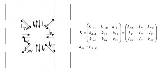
Figure 2.13 Implementation of a convolution kernel. The convolution kernel is realized by the current distribution from the pixel whose value is 1. Each current amount takes one of the three values,  $I_{ref}$ , 0,  $-I_{ref}$  where  $I_{ref}$  is the amount of the reference current. Only at the center pixel is allowed to have the value of  $2I_{ref}$  in addition to the above three values.
