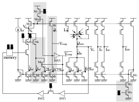
Figure 5.4 Pixel circuit schematic modified to accelerate the process of charging and discharging for the critical node  $N_{c}$ .
