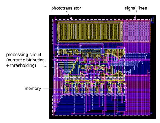
Figure 5.16 Layout of the pixel.
