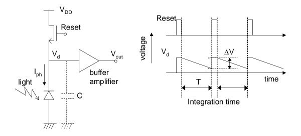
Figure 3.2 Schematic explaining the process of phototransduction. The node voltage  $V_d$ , which is first precharged to  $V_{DD}$ , starts decreasing after Reset is set low due to the discharging by the photogenerated current.
