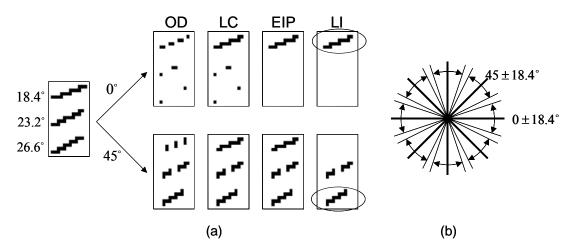
Figure 2.23 Schematic explaining the orientation tolerance of the proposed algorithm. (a) Result of the orientation decomposition followed by the three steps of subsequent processing. (b) Orientation range to be classified as one of the four orientations.
