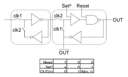
Figure 5.15 Schematic of the shift register. clk1 and clk2 are non-overlapping two phase clocks. Data transfer occurs when Reset is logic Low and Set^ is logic High. Actions for other switch settings are described in the table.
