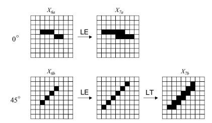
Figure 2.24 Line elongation operation and line thickening operation explained for  $0^{\circ}$  and  $45^{\circ}$  orientations.
