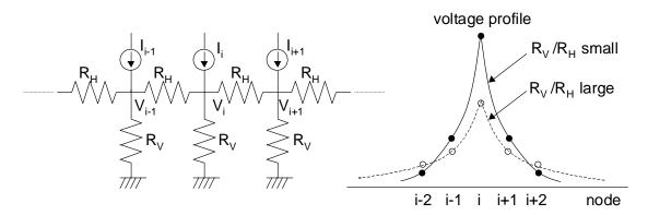
Figure 3.5 Resistive grid (left) and its impulse response (right). The impulse response is defined as the voltage profile for a current injected at one node. The voltage exponentially decreases as a function of distance from the node of current injection. The spread is larger for larger values of  $R_V/R_H$ .
