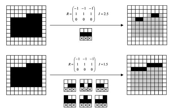
Figure 2.9 Orientation detection using template matching. The rectangular input pattern is used instead of line drawing patterns to demonstrate the selectivity of the template for the top edge and the bottom edge.
