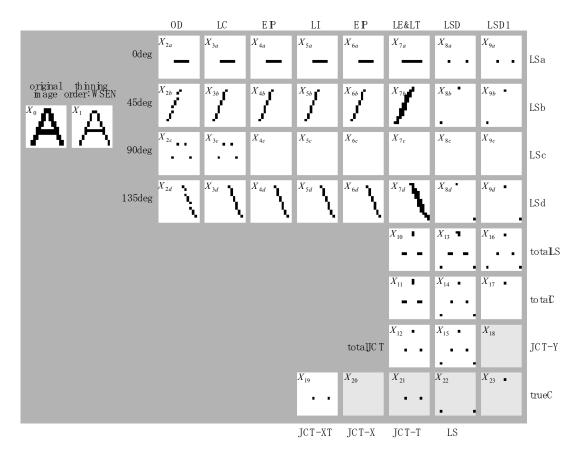
Figure 2.14 Overall processing flow of the feature detection algorithm. Features are detected by going through several processing steps. These steps include: OD (orientation decomposition), LC (line completion), EIP (elimination of isolated points), LI (line inhibition), LE (line elongation), LT (line thickening), and LSD (linestop detection). The detected features are: JCT-X (X-type junction), JCT-T (T-type junction), JCT-Y (Y-type junction), trueC (corners), and trueLS (linestops).
