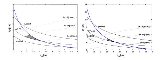
Figure 4.13 Relationship between the channel length and the reference current to ensure the transistor operation in the saturation region. The requirement is plotted as a thick line superimposed on the relationship shown in Figure 4.12. All the plots were made for the channel width of  $0.9 \,\mu\text{m}$ .
