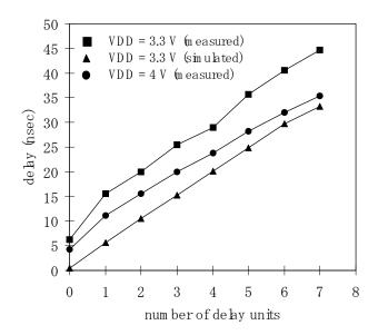
Figure 5.19 Measurement result of the delay of  $\phi_{2d}$  with respect to  $\phi_2$  for two power supply voltages ( $V_{DD} = 4 \text{ V}$  and  $V_{DD} = 3.3 \text{ V}$ ).
