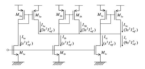
Figure 4.4 Current summation circuit. Note that there is no correlation between three currents  $I_{3a}$ ,  $I_{3b}$ , and  $I_{3c}$ . Expression in a parenthesis represents the variance of the current shown above the parenthesis.
