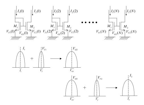
Figure 4.3 Schematic showing the increase of the current variation by current mirror operation.
