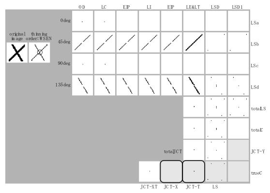
Figure 2.32 Simulation results for slanted letter "X". The vertical line segment (shown in the circle) generated by thinning leads to the detection of the T-type junction instead of the X-type junction (shown in the rectangle with a thick boundary).
