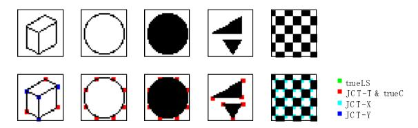
Figure 2.35 Features detected for various patterns. From left to right, they are indicated as wire frame of the rectangle, open circle, closed circle, closed triangles, checkerboard pattern.
