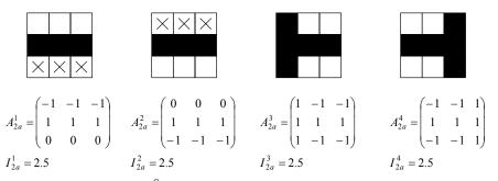
Figure 2.17 Patterns categorized as  $0^{\circ}$  with its corresponding template and threshold.
