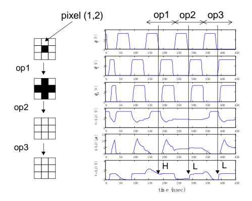
Figure 5.9 Simulation results at the clock frequency of 10 MHz using the circuit shown in Figure 5.7 with the delay between  $\phi_{2d}$  and  $\phi_2$  set to 5 nsec. An error was observed for *op1* operation at the pixel (1,2). The voltages and the current shown on the right-hand side represent those at the pixel (1,2).
