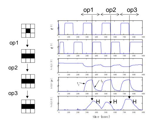
Figure 5.3 Simulation results at the clock frequency of 5 MHz. An error is observed at the center pixel during *op2* operation. The center pixel is still logic High although it should be classified as logic Low. The voltages and current on the right-hand waveforms represents those at the center pixel.
