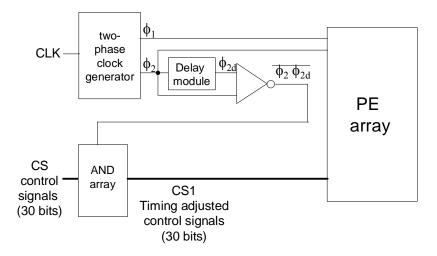
Figure 5.11 Schematic of the timing control circuit.
