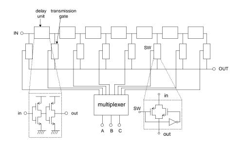
Figure 5.13 Circuit diagram of the programmable delay generator. One of the multiplexer outputs is set to logic Low to turn on the transmission gate and hence to connect the output of the selected delay unit to the OUT terminal. Each delay unit consists of two inverters.
