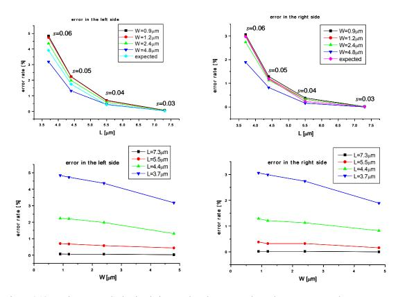
Figure 4.10 Hspice Monte-Carlo simulation result. The two graphs at the top represent the error rate as a function of the transistor channel length. The two graphs at the bottom represent the error rate as a function of the channel width. For these two cases, the graph on the left side and on the right side corresponds to  $p_{left}$  and  $p_{right}$ , respectively.
