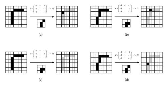
Figure 2.11 Schematic explaining the difficulty of corner detection using a  $3 \times 3$  template. In (a) and (b), the corner is correctly detected with different templates. When the combination of the pattern and the template is changed as shown in (c) and (d), no corner is detected in (c) and misclassification occurs in (d).
