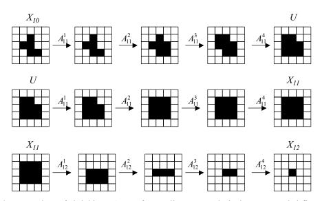
Figure 2.25 Procedure of shrinking. A set of mutually connected pixels are expanded first to form a circumscribing rectangle. Then the formed rectangle is shrunken to a single pixel.
