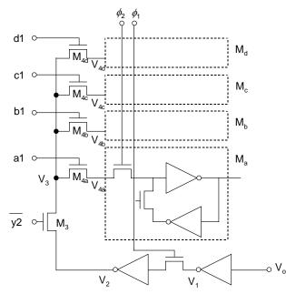
Figure 5.20 Schematic showing the signal transfer from the thresholding node to the memory. This figure is an extracted version from Figure 3.9 focusing on the memory configuration.
