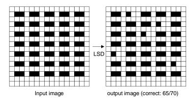
Figure 5.23 Schematic explaining the detection error for the linestop detection (LSD) operation. The output image shown in the right-hand half is one of the possible output images for an input image shown in the left-hand half. In this case, 65 pixels out of 70 pixels are correctly detected as linestops, indicating the error rate of 5/70.
