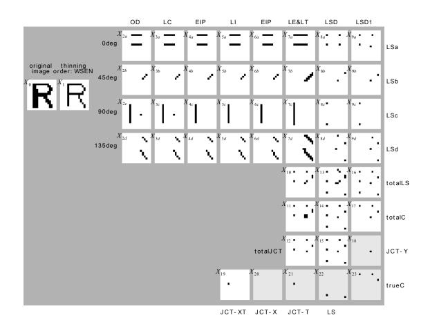
Figure 5.28 Detail of the processing flow for the letter "R".
