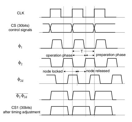
Figure 5.10 Modified timing diagram incorporating the delay signal  $\phi_{2d}$ . When  $\phi_2$  is logic Low, the operation is performed; when  $\phi_2$  is logic High, the precharging of the critical node is performed. The thresholding node is kept to  $V_{DD}/2$  while  $\phi_{2d}$  and  $\phi_2$  are both high.
