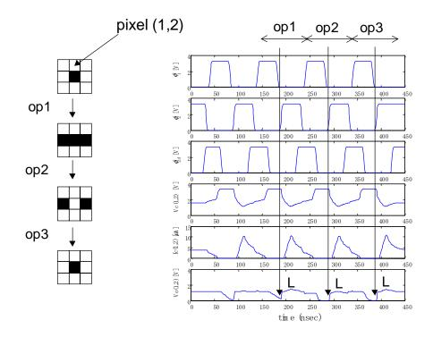
Figure 5.8 Simulation results at the clock frequency of 10 MHz using the circuit shown in Figure 5.7 with the delay between  $\phi_{2d}$  and  $\phi_2$  set to 30 nsec. All the operations are executed correctly. The voltages and the current shown on the right-hand side represent those at the pixel (1,2).
