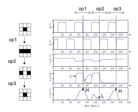
Figure 5.2 Simulation results at the clock frequency of 2.5 MHz. The evolution pattern is shown on the left. The top two waveforms correspond to a two-phase clock ( $\phi_1$  and  $\phi_2$ ). The third, fourth, and fifth waveforms represent the critical node voltage V<sub>c</sub>, the current output of the pixel I<sub>c</sub>, and the voltage at the thresholding node V<sub>o</sub>, respectively.
