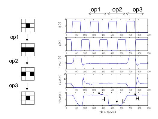
Figure 5.5 Simulation results at the clock frequency of 5 MHz using the modified circuit incorporating the high speed charging/discharging mechanism. All the operations were executed correctly. The voltages and the current on the right-hand waveforms represent those at the center pixel.
