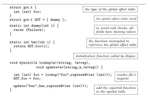
Fig. 4. Compilation of dynamically loadable code
