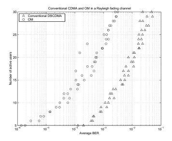
Fig. 5. Conventional DS-CDMA system and its OM counterpart. At  $PEP = 10^{-1}$  user capacity is doubled (BPSK spreading modulator with spreading gain K = 32,  $SNR := P/\eta = 0$ db).
