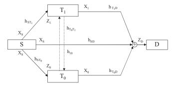
Fig. 1. Terminals  $T_0$  and  $T_1$  take turns in cooperating with S.
