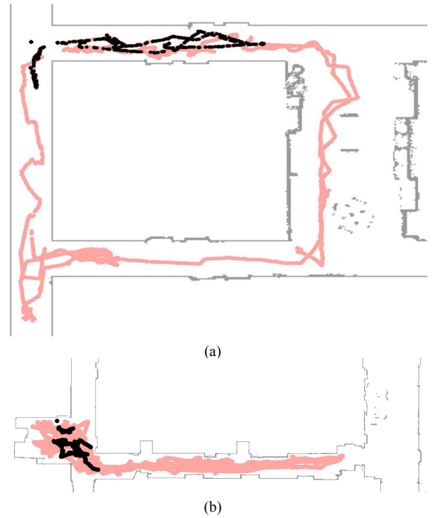
FIGURE 4. Local training locations. The local training set \mathbf{Y}_T is determined for (a) Levine and (b) Towne buildings by choosing 2% of the measurements in a subset of the environment—displayed here as black points.
