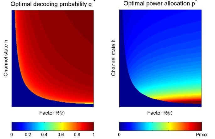
Fig. 6. Optimal decoding probability and power allocation for a FEC code. Color intensity indicates the magnitude of optimal decoding probability  $q^*$  and optimal transmit power  $p^*$  as functions of the factor  $R(\varepsilon)$  and the channel state  $h$ .
