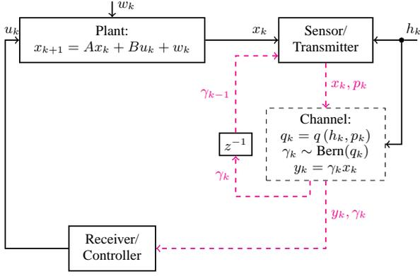
Fig. 1. Wireless control system architecture. A sensor measures the plant and wireless fading channel states  $x_k$ ,  $h_k$  respectively and transmits with power  $p_k$ . Messages are successfully decoded at the controller with probability  $q_k$  that depends on the channel state  $h_k$  and the power  $p_k$ . The sensor receives acknowledgments with a one-step delay.
