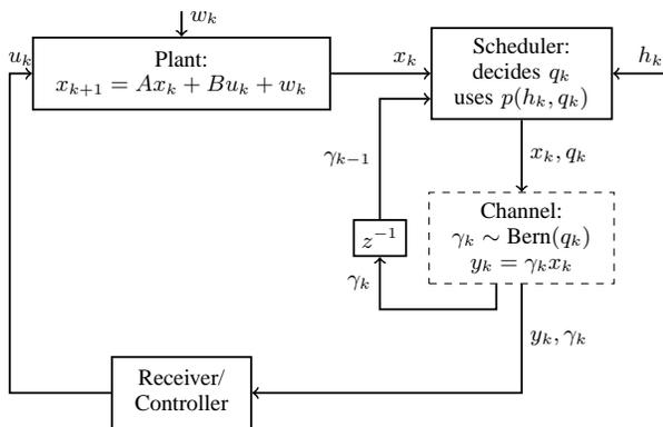
Fig. 3. Equivalent wireless control system architecture. A scheduler decides the successful decoding probability  $q_k$  and transmits the state measurement  $x_k$  with the required power  $p_k = p(h_k, q_k)$ . The controller receives the message with probability  $q_k$ .
