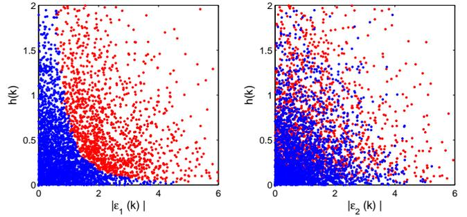
Fig. 7. Simulation results of the rollout policy for a capacity achieving code. The points  $|\varepsilon_{k,1}|, h_k$  and  $|\varepsilon_{k,2}|, h_k$  are plotted respectively, with blue indicating the decision to not transmit,  $q_k = 0$ , and red to transmit,  $q_k = 1$ .
