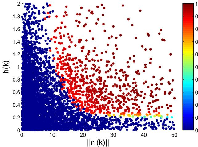
Fig. 9. Simulation results of the rollout policy for a FEC code. The points  $\|\varepsilon_k\|, h_k$  during the simulation are plotted with colors denoting the magnitude of the chosen decoding probability  $q_k$ . Practically  $q_k$  takes values either 0 or close to 1.
