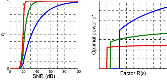
Fig. 5. Optimal power allocation for FEC codes with different complementary error functions. The optimal transmit power  $p^*$  is plotted as a function of the factor  $R(\varepsilon)$  for a fixed channel state  $h$  using FEC codes with different  $q$ -SNR characteristics. When the  $q$ -SNR curve becomes steeper, the optimal power allocation resembles a step function.
