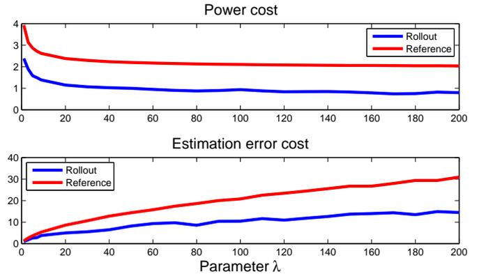
Fig. 8. Comparison of the optimal threshold policy and the resulting rollout policy performance for a capacity achieving code. The power and estimation error costs of the two policies are plotted for different values of the weighting factor  $\lambda$ . The estimation error cost for the reference increases at a faster rate than the rollout.
