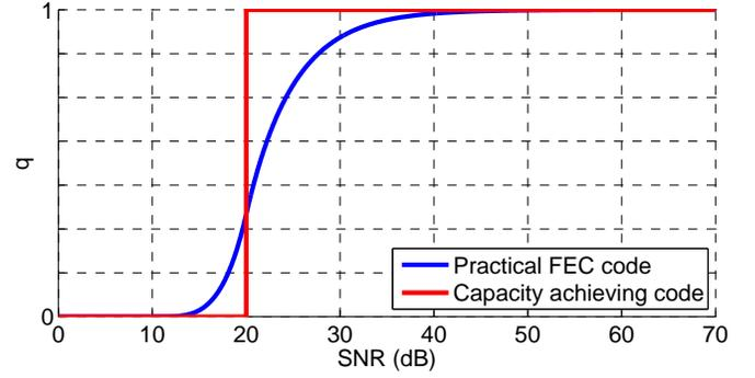
Fig. 2. Complementary error function for FEC and capacity achieving codes. The probability of successful decoding  $q$  for a practical FEC code is a sigmoid function of the received  $\text{SNR} = h p / N_0$ , while for a capacity achieving code a threshold value  $\text{SNR}_0$  determines whether a packet is successfully received.
