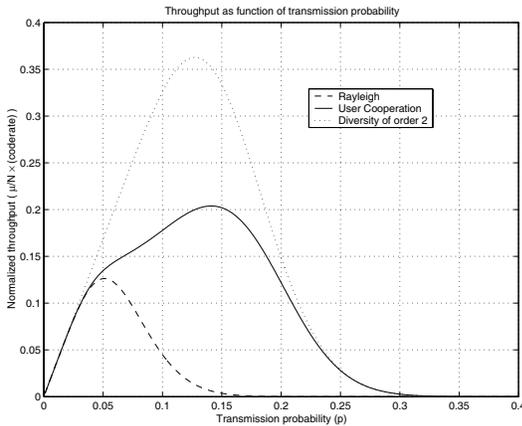
**Fig. 5.** Throughput of the CSSRA protocol lies in between the throughput of systems with and without diversity ( $J = 128$ ,  $N = 32$ ,  $L = 1024$ , 215/255 BCH code capable of correcting  $t = 5$  errors)
