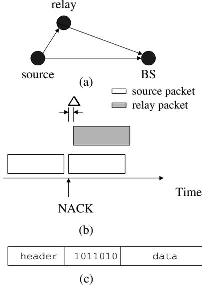
**Fig. 3.** (a) Each active user (source) receives cooperation from an idle user (relay); (b) When a packet is lost both source and relay transmit a copy of the packet; (c) Retransmissions occur at pre-specified randomly chosen time slots.
