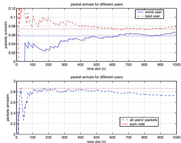
Fig. 9. Instances of the arrival rate processes for the max-min optimal routes in Fig. 8. The fairness of the protocol is manifested in the not so different rates offered to the best and worst nodes.
