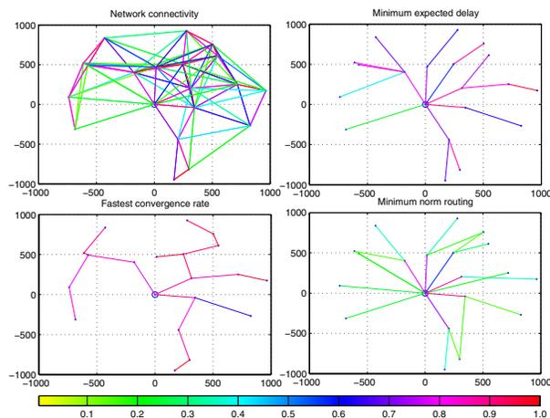
Fig. 3. A randomly generated network with 20 nodes, the color scale represents the elements of the matrix  $\mathbf{K}$ . Note how fastest convergence rate routing selects routes with large values of  $K_{ij}$ .
