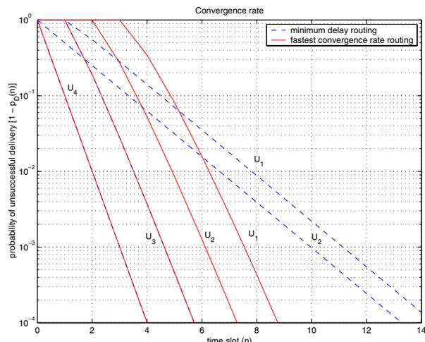
Fig. 2. Convergence rate for the network in Fig. 1. For a fixed time delay fastest convergence rate routing yields a smaller packet error probability.
