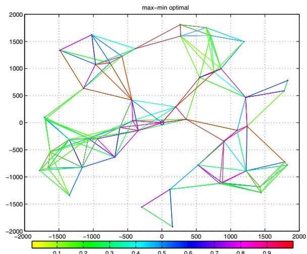
Fig. 8. Max-Min routes obtained as the solution of (24) for the network in Fig.6. Most nodes divide their traffic between many different neighbors to avoid the formation of bottlenecks.
