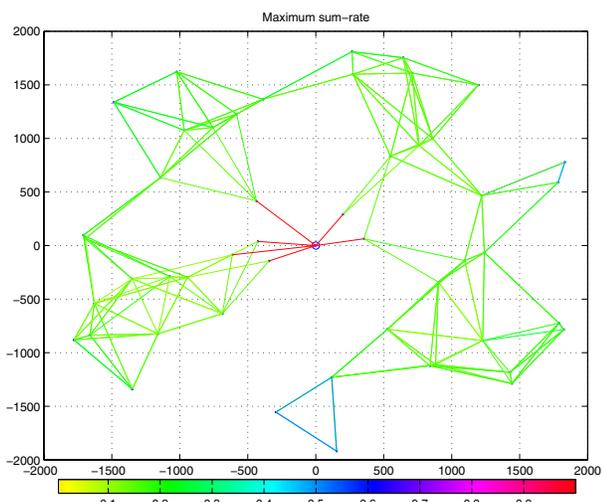
Fig. 7. Sum-rate optimal routes as given by (23). The nodes with good connections to the destination get most of the total rate available.
