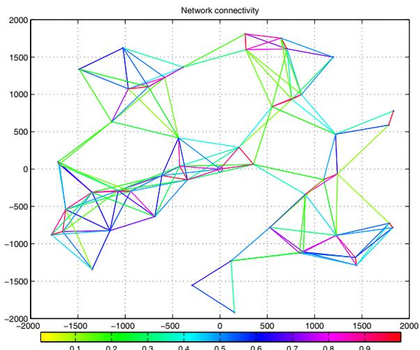
Fig. 6. Connectivity graph for a network with 50 nodes uniformly deployed in a circle with radius 2 Km, at whose center is the common AP. The color index represents the value of  $R_{ij}$  that is generated according to the empirical distribution in [7].
