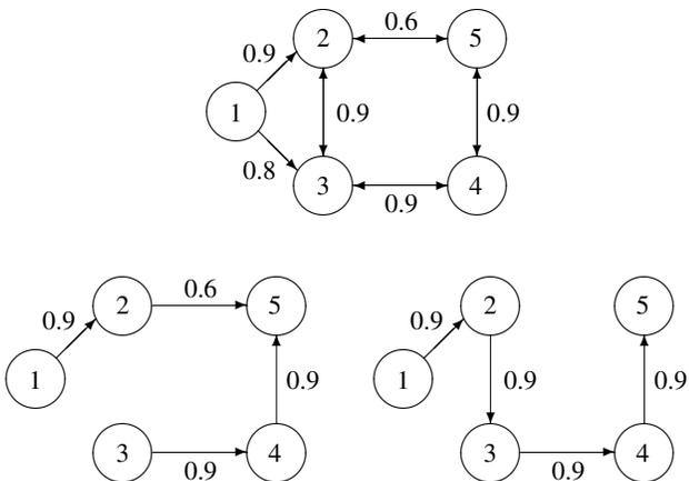
Fig. 1. For a simple connectivity graph (top,  $\mathbf{R}$  matrix shown) the minimum expected delay routing algorithm in (13) tends to select short routes (left, minimum expected delay  $\mathbf{K}$ ), while fastest convergence rate routing as per (8) selects longer routes with more reliable hops (right, fastest convergence rate  $\mathbf{K}$ ).
