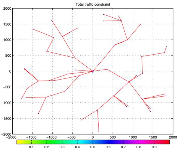
Fig. 10. Max-min routing with a global traffic limit as per (32). The routes are obtained as the shortest path in a fully connected graph with arc weights equal to  $1/R_{ij}$ .
