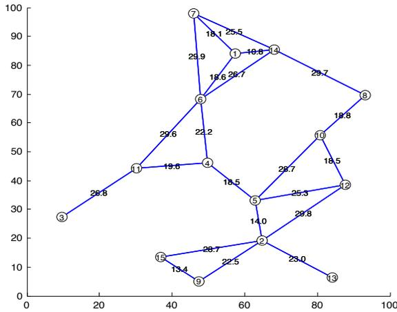
Fig. 3. Connectivity graph of a network used in simulation. The numbers on each edge shows the distance (in meters) between two communicating terminals.
