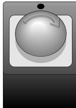
Figure 5-3. Emergency Stop Button
