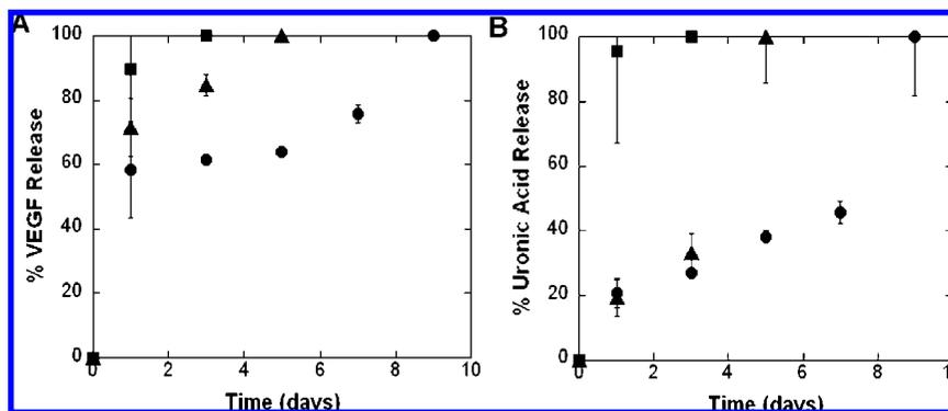
**Figure 2.** Degradation of hydrogels formed from MeLAHA macromers. VEGF (A) and uronic acid (B) release from pure MeLAHA hydrogels ( $n \sim 3.0$ , modification  $\sim 10.5\%$ ) at various macromer concentrations [ $\sim 1$  (■), 2 (▲), and 4 (●) wt%]. Both values are plotted as the cumulative percent release measured using quantitative analyses.
