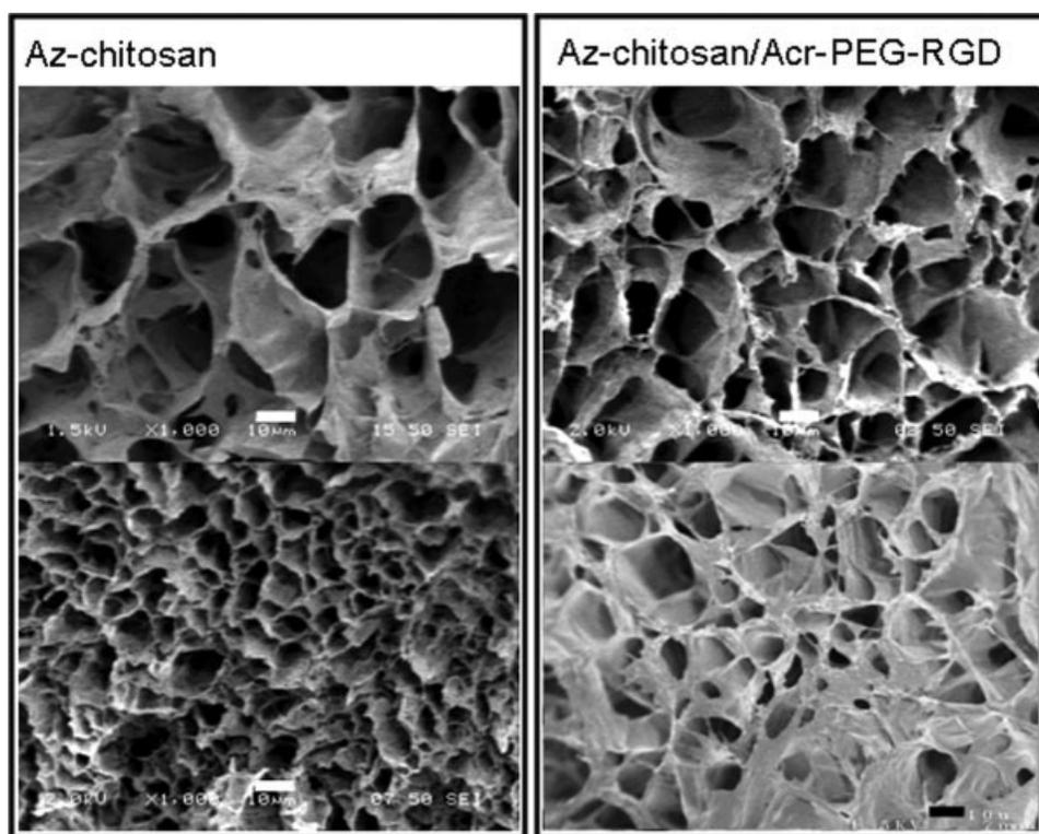
**Figure 2.** Scanning electron micrographs of lyophilized photocrosslinked gels. Two representative images were shown for each sample. Bars indicate 10  $\mu\text{m}$ .
