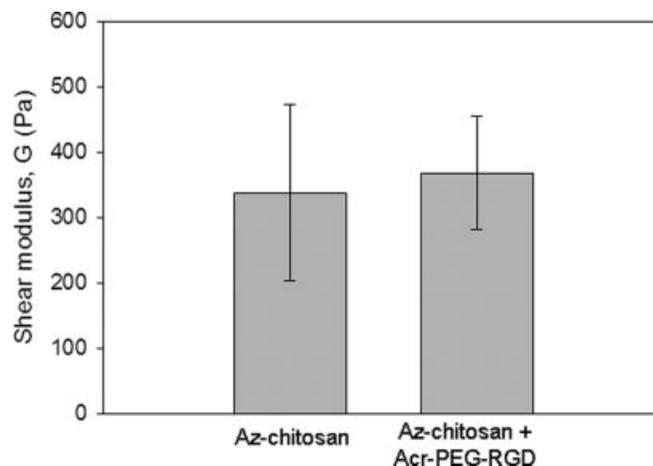
**Figure 1.** Mechanical properties of the hydrogels Az-chitosan and Az-chitosan/Acr-PEG-RGD hydrogel demonstrated comparable shear moduli. ( $N = 4$  per group).
