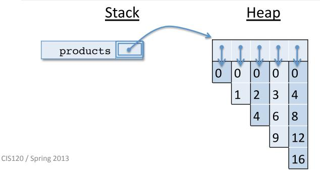
Note: This heap picture is simplified – it omits the class identifiers and length fields for all 6 of the arrays depicted.
