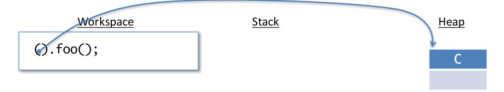
Allocate a new instance of C in the heap.
