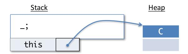
Save a copy of the current workspace in the stack, leaving a "hole", written \_, where we return to. Push the this pointer, followed by arguments (in this case none) onto the stack. Use the dynamic class to lookup the method body from the class table.
