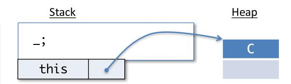
Save a copy of the current workspace in the stack, leaving a "hole", written \_, where we return to. Push the this pointer, followed by arguments (in this case none) onto the stack.
