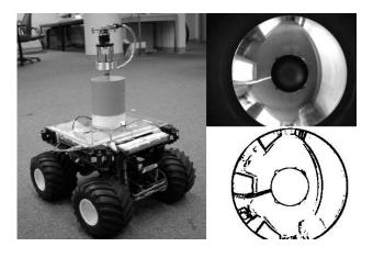
Figure 2: A Clodbuster robot and an image captured by the omnicam, before and after the edge extraction.
