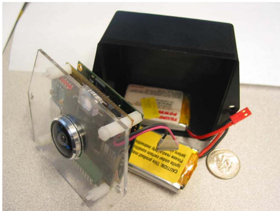
Fig. 2. Each smart camera module is equipped with an imager outfitted with a fisheye lens, a digital signal processor, an accelerometer, a CAN bus transceiver, and an LED signalling light
