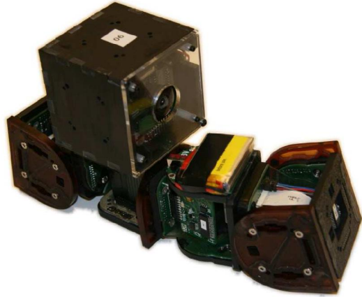
Fig. 1. Each cluster in the modular robot is composed of four CKBot modules and a smart camera system.
