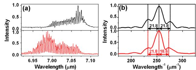
FIG. 1 (color online). (a) Spectra of a QCL with a 12- $\mu\text{m}$ -wide active region. (b) Fourier transform of the spectra. The laser is driven by pulsed current  $I = 1.0$  A (upper panel) and 0.75 A (lower panel) at a repetition rate of 80 kHz. The pulse duration is 125 ns.
