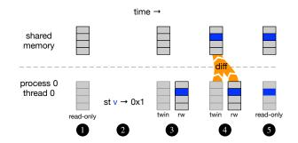
Figure 2: The Sheriff twin page mechanism.
