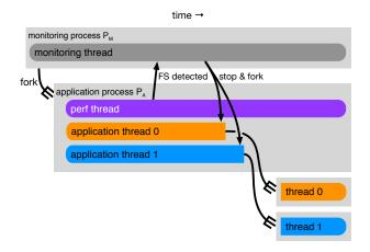
Figure 5: The process and thread organization of an application running with TMI.
