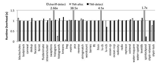
Figure 7: Performance of TMI's allocator and false sharing detection compared to sheriff-detect. All bars are normalized to pthreads execution using the Lockless allocator (lower is better). *TMI-alloc* redirects all memory alloctions to TMI's process-shared memory. *TMI-detect* enables all other necessary features of TMI's false sharing detector (Section 3).
