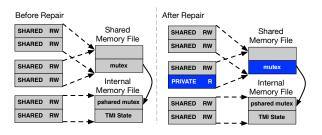
Figure 6: The shared memory layout before and after targeted repair with TMI as described in Section 3.2
