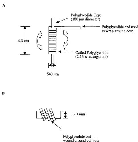
**FIGURE 1.** Diagram of a BPC. *A*, a 5-0 suture is wound around a core of the same size suture (5-0) to form the primary coil. *B*, the primary coil is then wound around a 3-mm-diameter cylinder to form the secondary coil.
