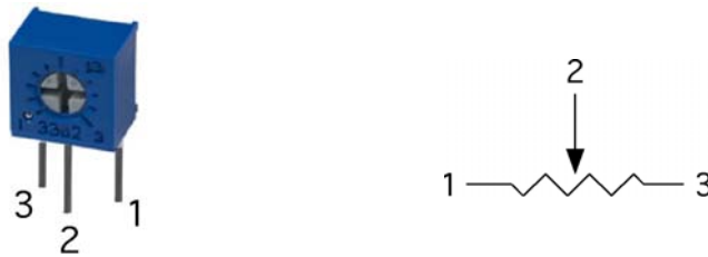
Figure 8 – Potentiometer (Left) and Circuit Representation (Right)
