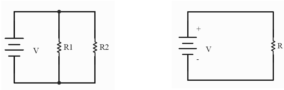
Figure 6. – Resistors in Parallel and Equivalent Circuit
