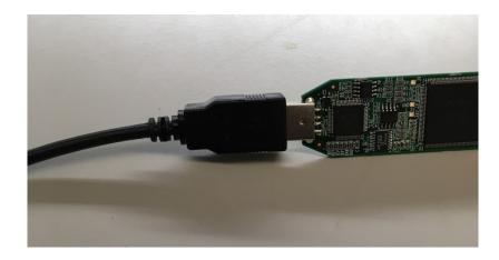
v. Lastly, connect the FPGA to the Linux computer (the smaller of the two Dell machines) at your lab station. Plug into the leftmost USB port on the main computer box.
