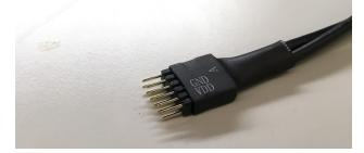
ii. Connect the Pmod buttons to the end of the Pmod extension cable that has 6 holes and is labeled A, and the Pmod switches to the other end. The buttons and switches should look as follows:
