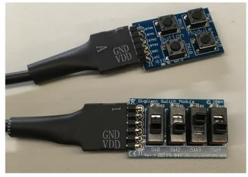
iii. Connect the Pmod extension cable with the male to male headers to the FPGA, such that the side labeled A faces **outward**:
