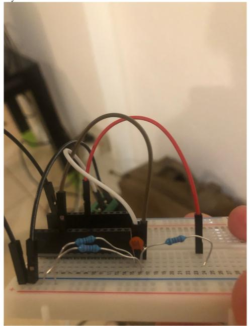
5. Finally, connect the audio input wire into the same row of the capacitor as the 1kOhm resistor. Connect the other side of the last 10K Ohm resistor to the USB pin of the Itsy-Bitsy, and connect the other side of the capacitor to pin A0. The final product should look like this:
