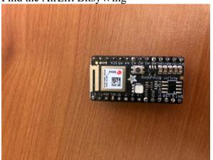
Note the antenna (shown on right in this diagram) is fragile. Use care not to put force on it when inserting and handling the AirLift.
