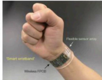
a) W. Gao, S. Emaminejad, H.Y.Y. Nyein, S. Challa, K. Chen, A. Peck, et al., Fully integrated wearable sensor arrays for multiplexed in situ perspiration analysis. Nature 529 , 509–514 (2016)
