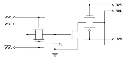
(a) Is this a SRAM or DRAM cell? Explain your reasoning? DRAM. The data is stored on a capacitive node and is not actively driven
