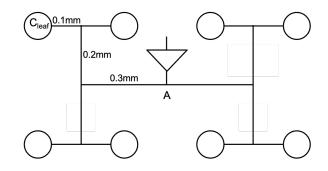
$C_{leaf}$  is the total capacitance for some number of clocked circuits in a region of the chip (we might just keep branching the clock tree until it gets down to a single output; for this problem we're building a small tree and lumping a group of circuits together at the leaf to keep the problem size small).
