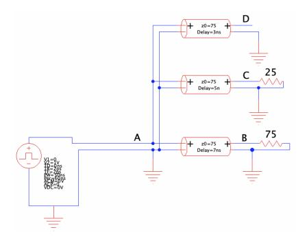
(a) Given the source waveform is a 1V step at 0ns (shown below), draw the expected waveforms seen at B, C, and D from 0ns to 30ns.
