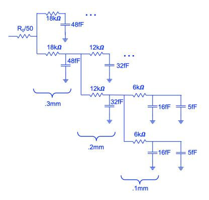
Using straight Elmore delay with lumped wire model, we can get the delay to any leaf node:
