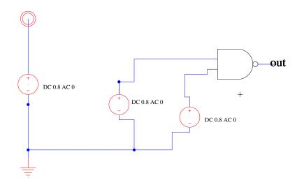
Set all the voltage sources to DC 0.8V. In general, parameterized schematic elements (like transistors and voltage sources) have properites associated with them that you may need to set. Here, the voltage supplies have both an AC and DC voltage parameter. Leave the AC parameter at 0. You can change the value by double-clicking on the value (not the cell). You can actually change the entire text here, but you should leave it with "DC 0.8 AC 0".
