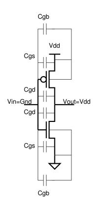
(a) What is charge, Q, on each of the capacitors when Vin=Vdd and Vin=Gnd? Pay carefull attention to polarities. (Qab = - Qba)
