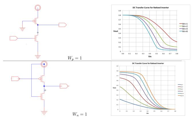
1. Size  $W_n$  or  $W_p$  for correct operation with  $V_{ol} \leq 0.1 V_{dd}$  and  $V_{oh} \geq 0.9 V_{dd}$ .
