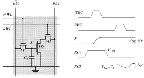
5. Below is the 1T DRAM cell with waveform for writing a '1' into the cell and then reading the cell.
