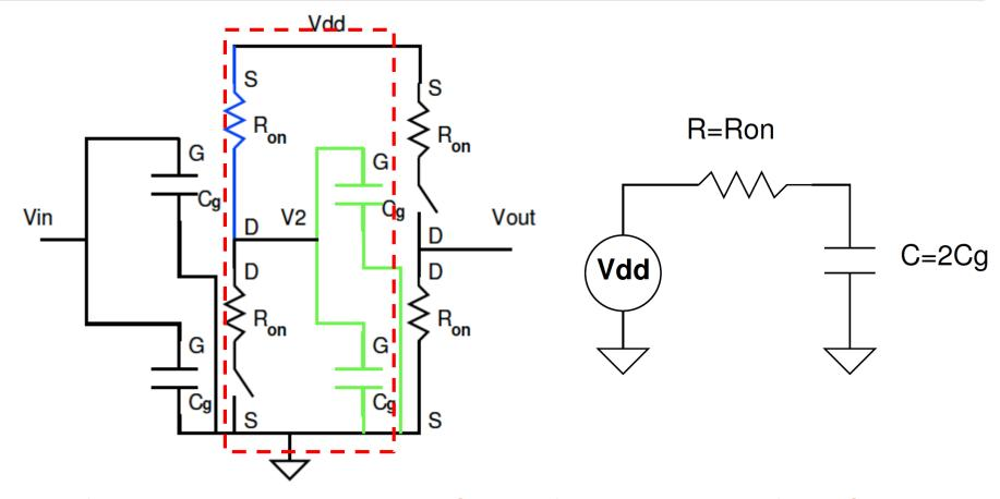
■ What is time constant of  $V_2$  when  $V_{in}$  switches from  $V_{DD}$  to 0?
