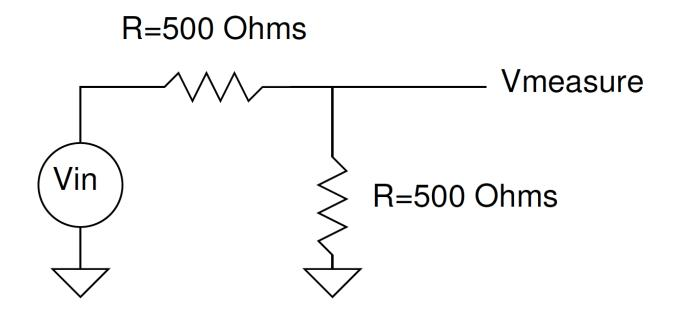
Assume  $V_{in}$  is 0 for t < 0 and steps to 1V at t = 0.
