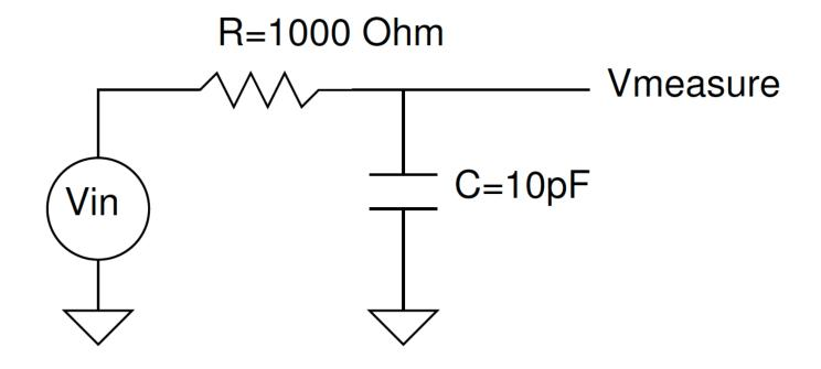
Assume  $V_{in}$  is 0 for t < 0 and steps to 1V at t = 0.
