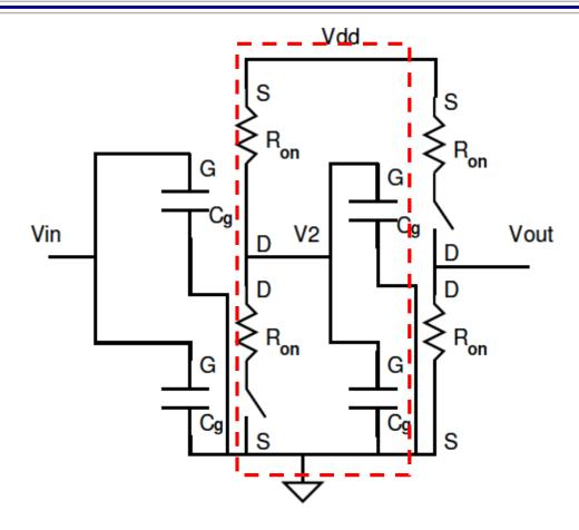
■ What is equivalent circuit for the gate output of stage 1 driving  $V_2$ ? What is load on the output of stage 1?
