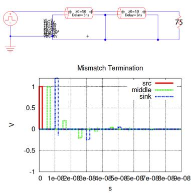
4. Transmission Line Termination Fill in the table below and match the following transmission line circuits (1-5) with the correct pulse propagation plot (a-d) for sending a pulse down the transmission lines to a resistive load. There is intentionally one less plot than circuit. The effective resistance seen into the source is a short circuit.
