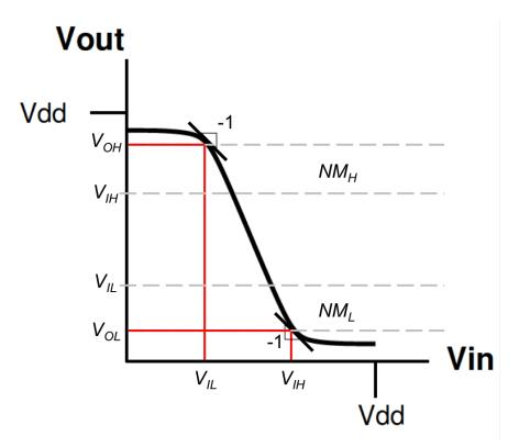
$$NM_H = V_{OH} - V_{IH} \tag{1}$$
