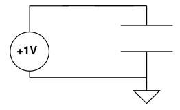
(b) Assume the capacitor has a capacitance of 1F, what is the charge on the top plate? What is the charge on the bottom plate?
