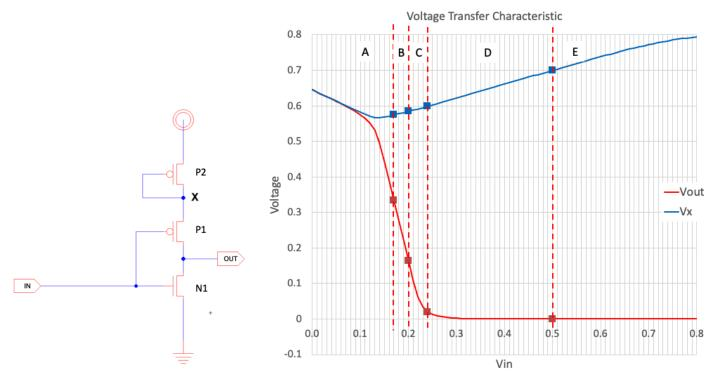
For the regions A-E labeled on the transfer function, identify the region of operation of the nMOS and both pMOS devices. Fill out the table below.
