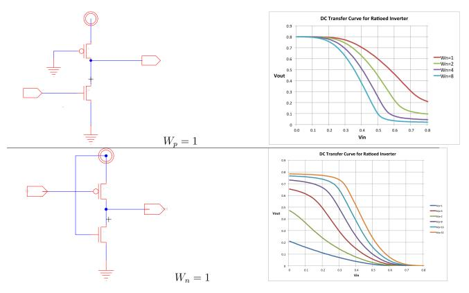
1. Size  $W_n$  or  $W_p$  for correct operation with  $V_{ol} \leq 0.1 V_{dd}$  and  $V_{oh} \geq 0.9 V_{dd}$ , where  $V_{dd} = 0.8$ . Assume extreme velocity saturation,  $R_{0p} = R_{0n}$ .
