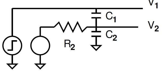
Spice: R<sub>2</sub>=1K, C<sub>1</sub>=10pF, C<sub>2</sub>=20pF ٧ı C₁ ି<sub>2</sub>  $R_2$ spice deck for cell test\_cap\_undriven{sch} from library 1 vict **V2** 0.9 aggress **V1** 0.8 0.7 0.6 diversion > 0.5 0.4 0.3 0.2 0.1 0 5e-08 1e-07 1.5e-07 2e-07 0 S
