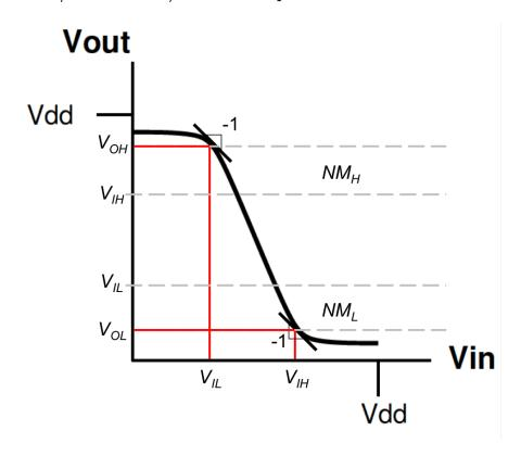
$$NM_H = V_{OH} - V_{IH} \tag{1}$$
