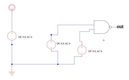
Set all the voltage sources to DC 0.8V. In general, parameterized schematic elements (like transistors and voltage sources) have properites associated with them that you may need to set. Here, the voltage supplies have both an AC and DC voltage parameter. Leave the AC parameter at 0. You can change the value by double-clicking on the value (not the cell). You can actually change the entire text here, but you should leave it with "DC 0.8 AC 0".
