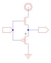
Assume:  $V_{dd}$ =0.8V,  $V_{thn}$ =250mV,  $V_{thp}$ =-250mV. Reason using your first-order transistor model.
