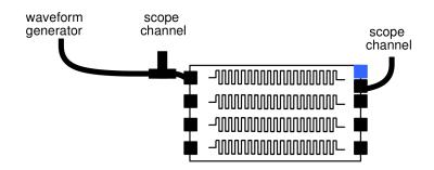
i. For what resistance do you see minimal or no reflection? Use the multimeter to measure the potentiometer resistance.
