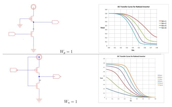
1. Size  $W_n$  or  $W_p$  for correct operation with  $V_{ol} \leq 0.1 V_{dd}$  and  $V_{oh} \geq 0.9 V_{dd}$ .
