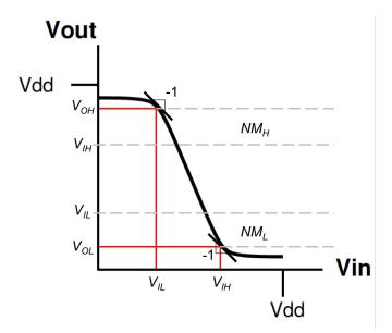
$$NM_H = V_{OH} - V_{IH} \tag{1}$$
