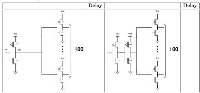
4. How should we size the transistors in middle stage?
