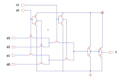
Report worst-case delay for the passT mux4 from the  $R_0$  input driver driving the inputs through driving the  $8C_0$  load on the output in units of  $\tau$ . Assume the same inputs drivers. Show individual stage delays for partial credit.
