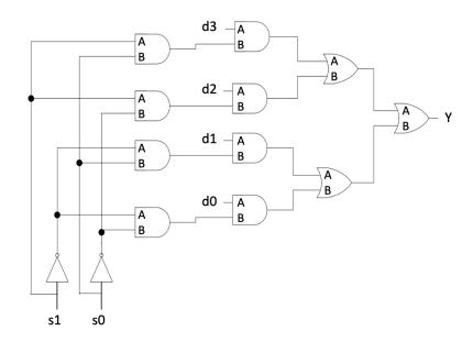
Report worst-case delay for the CMOS mux4 from the  $R_0$  input driver driving the inputs through driving the  $8C_0$  load on the output in units of  $\tau$ . Show individual stage delays for partial credit.
