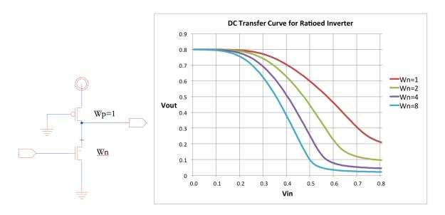
The IV curves indicate a  $W_n \ge 2W_p$  for noise margins within 25% for  $W_p = 1$ . Therefore sizing every stage should with  $\frac{R_0}{3}$  drive results in the following sizing.
