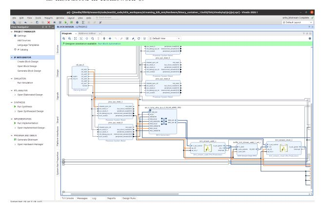
You can see from the vivado block diagram that clock index 1 is assigned. Moreover, you can also see that an AXI Stream FIFO is connecting the two kernels.
