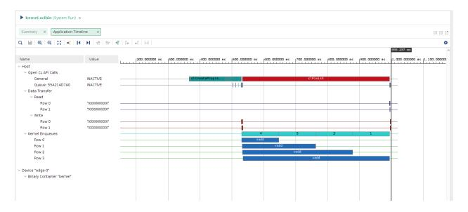
From the application trace, we can see that although the host scheduled all kernel executions concurrently, the second, third and fourth execution requests are delayed as there is only one compute unit on the FPGA.
