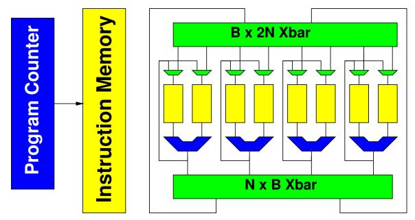
N is the number of physical ALUs. ALUs produce and consume w bits of data. Data memories local to each ALU store w-bit wide data. There are two data memories per ALU as shown. You can think of the Program Counter as being similar to the one from HW4. It should get inputs from the datapath and instruction memory, but we will assume we do not need model that any further than the area/energy model for the program counter shown below.
