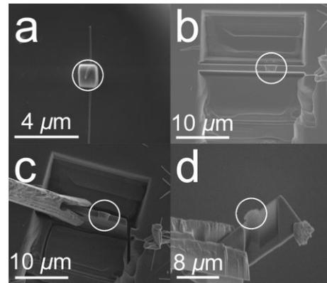
**Figure 4.** The FIB lift-out technique. The target area is circled in all four images. a) The target area is protected with a EBID-Pt capping layer. b) Trenches are cut on both sides of the target area. c) The micromanipulator is used to pick up the slab for further thinning. d) A side view of the slab shows that thinning has made the target area almost electron transparent.
