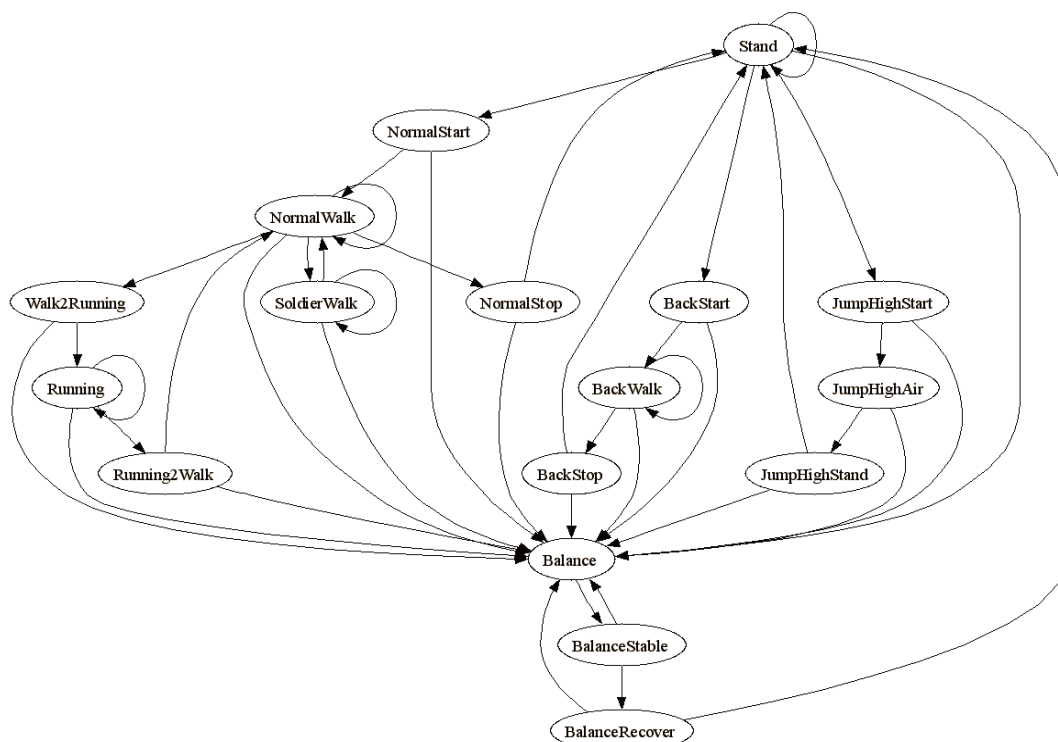
Figure 19. An example of finite state machines that govern transitioning between motor controllers. The nodes correspond to motor controllers and the edges show the transition possibilities between controllers.
