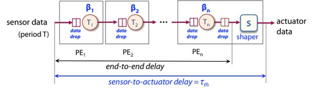
Figure 11: Buffer control mechanism for the platform.
