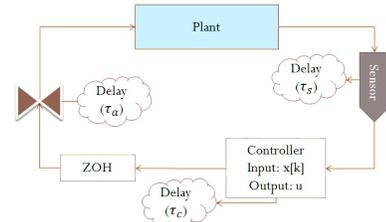
Figure 1: Schematic overview of the control of a plant using a DES.
