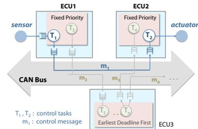
Figure 14: System architecture for the lane keeping system.
