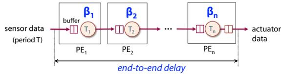
Figure 10: A platform architecture for a control system.
