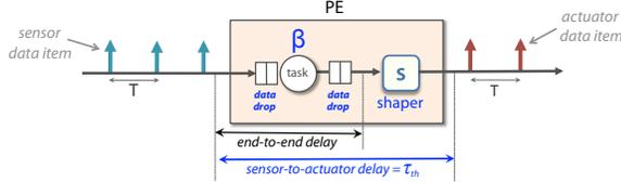
Figure 12: The transformed system that is used for the analysis.
