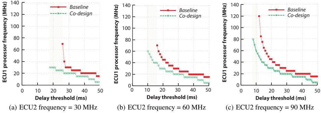
Figure 15: ECU1 processor frequency for different delay thresholds.
