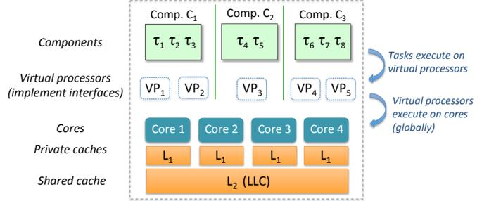
Fig. 1: A compositional system on a multicore platform. Here, the resource demands of tasks in a component are abstracted as an interface. This interface is further transformed into a set of virtual processors, which supply resources to the tasks of the component. The virtual processors of all components are globally scheduled (e.g., as servers) on the cores. Each core has a private cache, and all cores share a shared cache.
